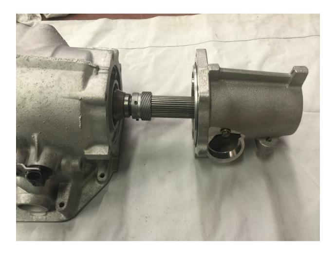
Install the drive gear with three set screws facing the front or towards the transmission. See Picture for proper orientation.
