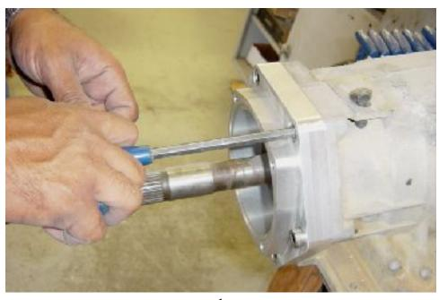
Install original o-ring on 6-bolt adapter. Position adapter on transmission and secure with six stainless cap screws.
