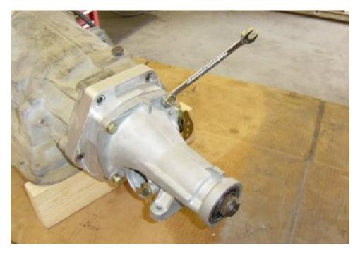
Install tail housing with supplied four bolts.
