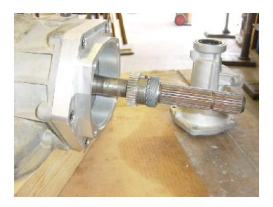
Slide reluctor/drive gear assembly onto output shaft. Do not tighten/set screws. Approximate reluctor/drive gear assembly, so that drive gear is in the center of speedometer sleave opening.
