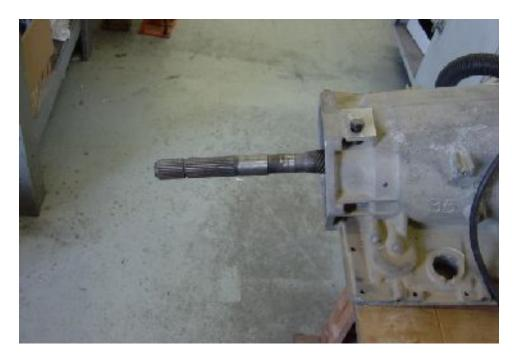
Remove original tail housing and reluctor gear and sleeve. There should be nothing on the output shaft. Retain tail housing o-ring to use on adapter.
