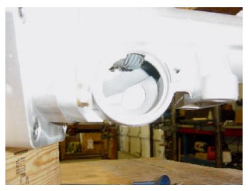
Install tail housing onto adapter with 4 bolts and tighten. Position reluctor/drive gear assembly, so that drive gear is in the center of speedometer sleave opening.
