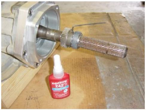
Loosen 4 tail housing attachment bolts and remove tail housing. Take care not to move reluctor/drive gear assembly while removing tail housing. Use Loctite 242 on the three set screws and tighten until secure.
