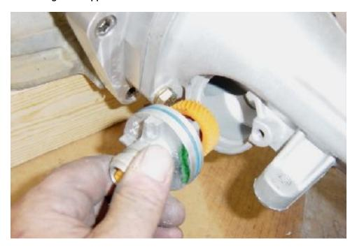
Remove speedometer sleave clamp and install sleave. Install clamp, taking care to position sleave so clamp tangs fit into the sleave properly. Hook-up VSS sensor and mechanical speedometer cable.
