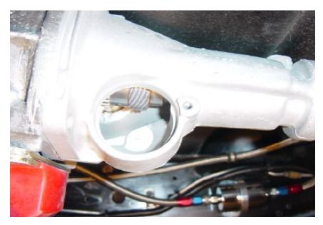
Remove extension housing. Being careful not to move the reluctor gear/ drive gear assembly, tighten the three set screws with an allen wrench to secure assembly to output shaft. Install extension housing onto transmission, fasten with bolts, and tighten evenly.
