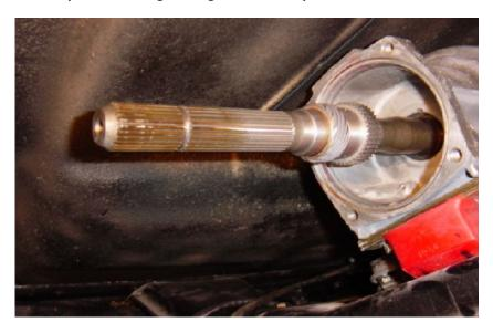
Slide tail housing into transmission until seated and visually confirm that the drive gear of the assembly is centered in sleeve opening. See picture below.
