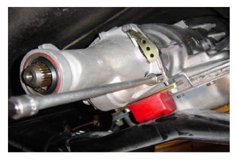
Install sleeve assembly into extension housing opening. Secure sleeve into extension housing with clamp and bolt provided. This completes extension housing installation.
