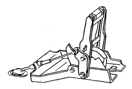
Kits convert the factory Automatic console shifter to OverDrive Operation with all gears available. Some of the **4LxxE** Series transmissions use a Long Range Select Shaft to add an external Neutral Safety Switch to the Transmission. Use of the longer shaft requires a non-offset lever, included in this kit. SHIFTWORKS®.
