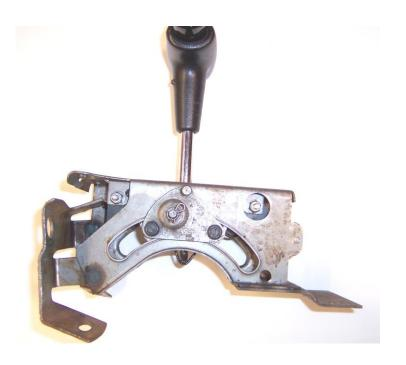
1. Remove the **cable mount** from the side of the shifter and replace with the one supplied. **(For 6-speed conversions, skip step #2)**
