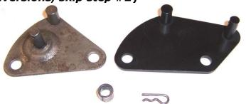
2. Remove factory detent from shifter housing and install your new Shiftworks detent using the supplied 10-24 x 3/4" machine screws and lock nuts.
