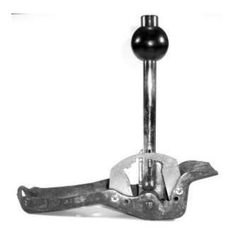
KITS CONVERT THE FACTORY AUTOMATIC SHIFTER TO FUNCTION PROPERLY WITH A NEW OVERDRIVE TRANSMISSION WITH ALL DETENTS AVAILABLE. USE WITH SHIFTWORKS CABLE #K102-29 OR FACTORY CABLE GM#3958079 (68-76) OR GM#357746 (77-81). KITS INCLUDE NEW DETENT, CABLE INSTALLATION HARDWARE, INDICATOR PLATE, AND INSTRUCTIONS.
