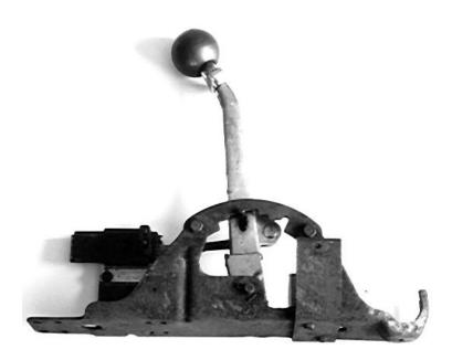
KITS TO CONVERT THE FACTORY CONSOLE SHIFTER TO CABLE OPERATION WITH ALL DETENTS AVAILABLE.
