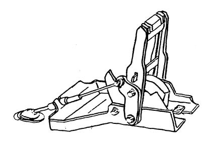
Kits convert the factory Automatic console shifter to OverDrive Operation with all gears available.
