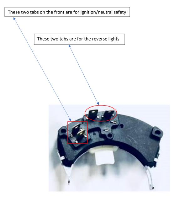
**NOTE:** The switch is a simple circuit interrupt. There is no special in or out for each pair of contacts
