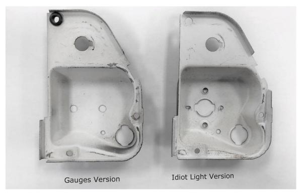
GM used the same metal pod for the Ammeter as they did for the Idiot Light. However, the back of the housing was punched differently. You can simply modify the back as described below.
