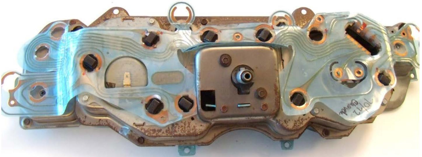
Remove the plastic circuit board from the rear. Be careful not to damage it. If not replacing the clock with our tachometer you may leave the center section attached.
