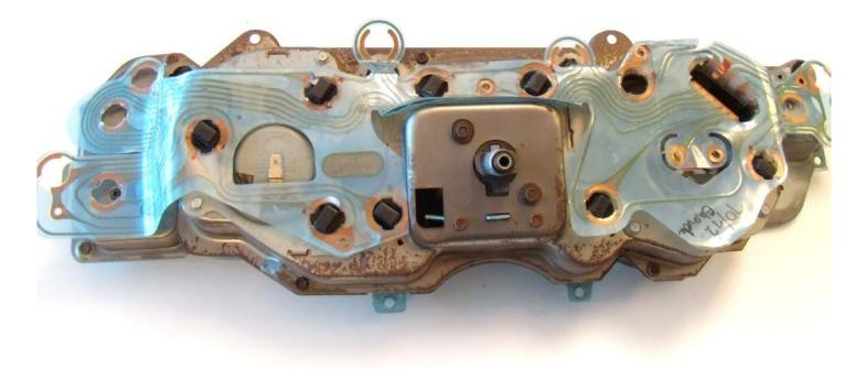
Remove the plastic circuit board from the rear. Be careful not to damage it. If not replacing the clock with our tachometer you may leave the center section attached.
