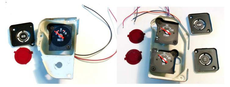
Remove idiot light covers and install gauges. Thread the wires out the back.
