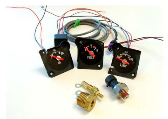
The S511 kit includes an Electrical Oil Pressure Gauge, a Voltmeter and an electric Water Temperature gauge. You will re-use the idiot light mounts so do not damage them as they are removed.
