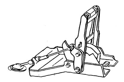
Kits convert the factory Automatic console shifter to 3-Speed Operation with all gears available
