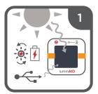
Charge outside in direct sun for 10 hours. Charge by micro-USB input for 1-2 hours. Red LED indicates battery is charging.
