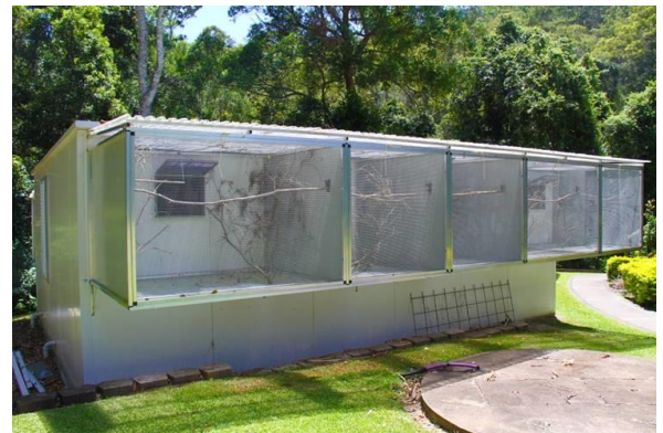
Aviary Complex constructed of refrigeration panels
