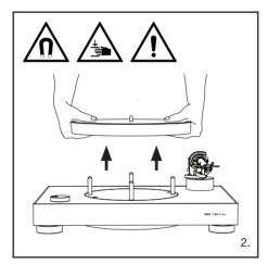
Hold the levitating platter firmly with both hands and remove it by lifting it vertically.
