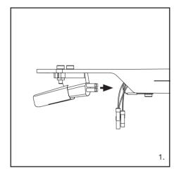
Remove the lead wires. Be careful not to damage the lead wires.
