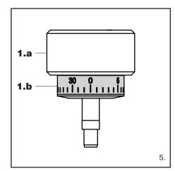
While supporting the counterweight so that it does not move, turn the tracking force gauge ring so that its "0" position lines up with the centerline on the back of the tonearm (the tracking force is not adjusted simply by turning the tracking force gauge ring).
