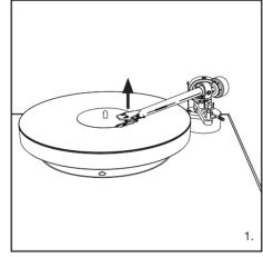
30 seconds after the tonearm reaches the end of the record, the tonearm will lift itself and the levitating platter will slowly stop rotating.
