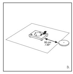
Make sure to place the removed levitating platter at least 50cm (20") away from the turntable body and away from any metal, magnetic or electronic objects, to avoid damage to the apparatus or other possessions.
