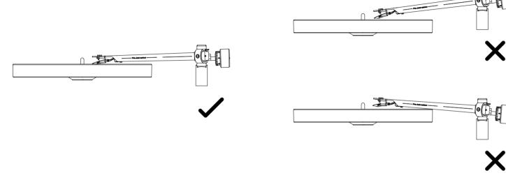
As you can see there are two different angles serving the same purpose. VTA and SRA. These angles are affected by the height of the tonearm and tracking force. The height of the tonearm raises the actual pivot point of the cantilever
