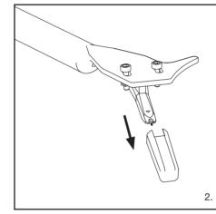
Remove the cartridge's protector, by pulling straight forward. Applying a downward force may cause the stylus to come off the body. Only low volume is output if the stylus has come off, or is about to come off, so refer to "Replacing the stylus" (page 34) to reattach the stylus correctly.
