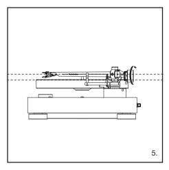
Turn the counterweight until the tonearm is parallel to the platter.
