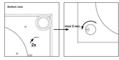
1. Press the reset button on the bottom of the turntable body two times, quite fast (inside the span of 1 second).
