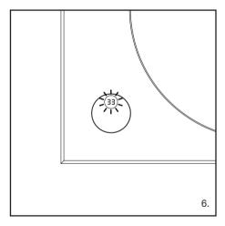
When the levitating platter reaches the correct speed and stabilizes, the light in control button will stop blinking and the tonearm will lower itself and place the stylus on the record.
