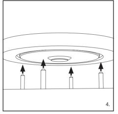
The platter feet will automatically rise and hold the levitating platter.
