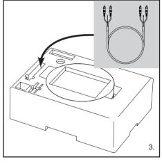
Take out the RCA cables and remove the ties.
