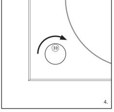
Turn the control button clockwise from OFF mode (9 o'clock), to 33 (33.3 rpm – 12 o'clock) or 45 (45 rpm – 3 o'clock), depending on the speed the record is supposed to be played at. This turntable only plays 33.3 rpm and 45 rpm records.
