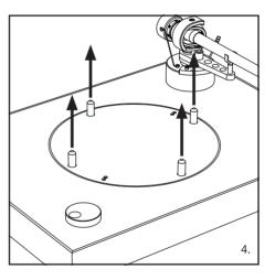
When the turntable is plugged into the electric power grid for the first time, the platter feet will rise out of the turntable body into set up position.
