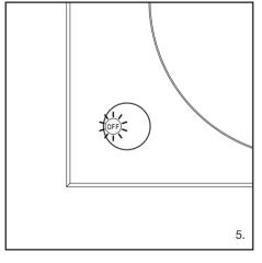
When the light in the control button stops blinking, the turntable body set up is finished.
