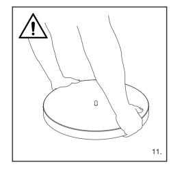
When taking out or handling the platter, grip with both hands and always keep it away from any metal or magnetic object, cellphones, tvs or any other electronic equipment. (minimum 50cm or 20" distance)
