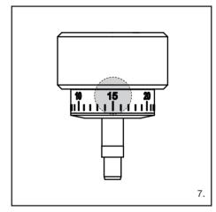
Let go of the downforce scale and rotate the counterweight between 15-16 (for Ortofon OM10).
