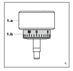
Adjust the tonearm balance and tracking force. Refer to "Tonearm balance and tracking force (page 20) to perform the readjustments."
