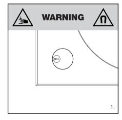
Make sure the control button is in OFF mode, platter feet are raised and the levitating platter is resting solidly on the platter feet.
