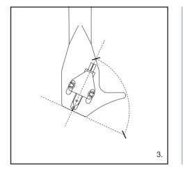
Using a commercially sold, non-metallic slotted screwdriver, tighten the screws in both places, and then adjust the overhang. After the adjustments are complete, tighten the screws securely.
