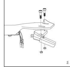
Using a commercially sold, non-metallic slotted screwdriver, remove the installation screws, and then remove the cartridge from the headshell.
