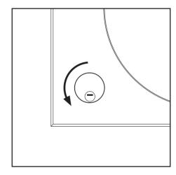
Make sure the turntable is set up propperly. Turn the control button counter-clockwise to – mode (6 o'clock).
