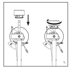
With the tracking force gauge ring facing forward attach the counterweight to the back of the tonearm, and slowly turn it counterclockwise (to the left)
