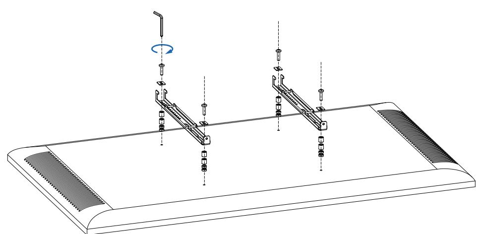
EN Select appropriate screws from M-A to M-G and install part # 4 on the four screw holes on the back of the TV. The back of the TV is flat, and the A1 installation method without gasket can be used; If the back is uneven, A2 installation method with washers (M-H to M-J) can be used, and thick washers can be superimposed according to the situation.
