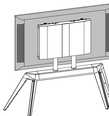
**EN** Use a 6mm Allen wrench to adjust the TV backplane to a proper height.
