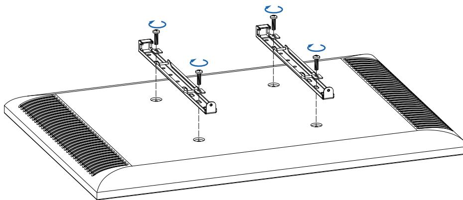
**EN** Select appropriate screws from M-A to M-G and install part #7a on the four screw holes on the back of the TV. The back of the TV is flat, and the **A1** installation method without gasket can be used; If the back is uneven, **A2** installation method with washers (M-H to M-J) can be used, and thick washers can be superimposed according to the situation.
