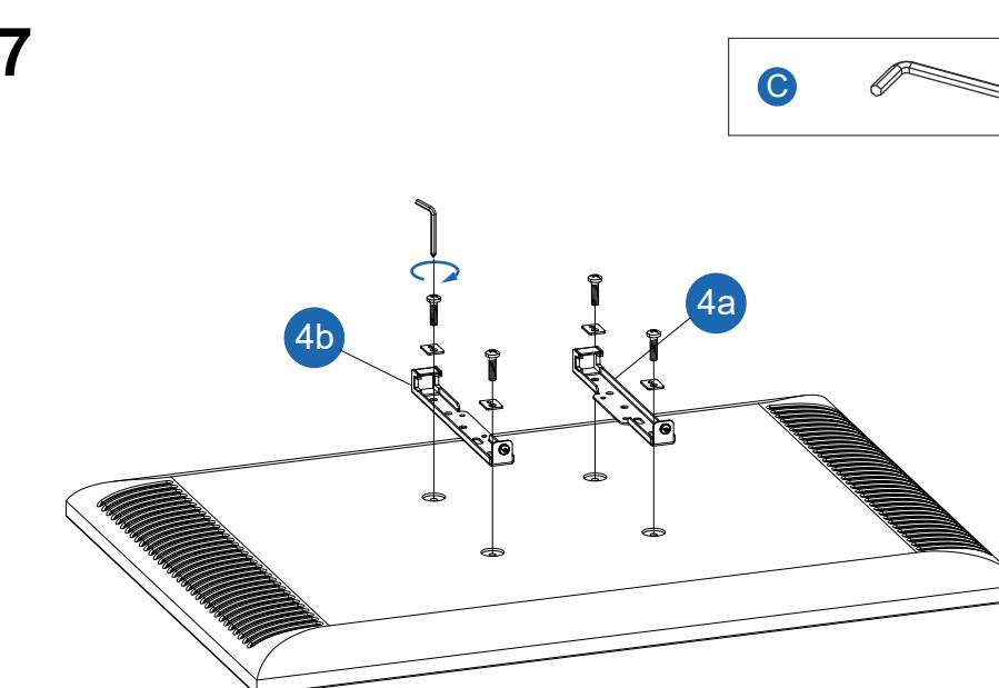
**EN** Select appropriate screws from M-A to M-G and install part # 4 on the four screw holes on the back of the TV. The back of the TV is flat, and the **A1** installation method without gasket can be used; If the back is uneven, **A2** installation method with washers (M-H to M-J) can be used, and thick washers can be superimposed according to the situation.
