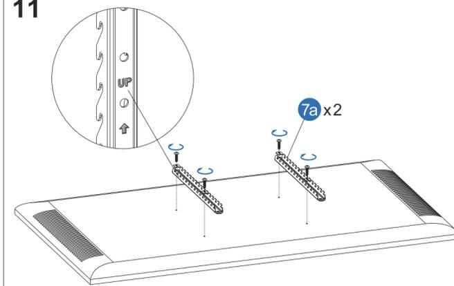
Select appropriate screws from M-A to M-G and install part #7a on the four screw holes on the back of the TV. The back of the TV is flat, and the A1 installation method without gasket can be used; if the back is uneven, A2 installation method with washers (M-H to M-J) can be used, and thick washers can be superimposed according to the situation.
