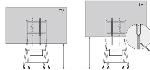
The adjustable range of the distance from the bottom of the TV to the ground is marked on the part 7, so that you can choose the appropriate height. You can choose the height, make a mark on the ruler, and then disassemble and install the part 7 to the back of the TV.
