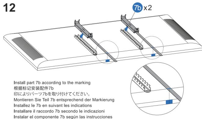
Install part 7b according to the marking
