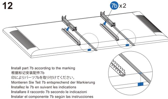
Install part 7b according to the marking
