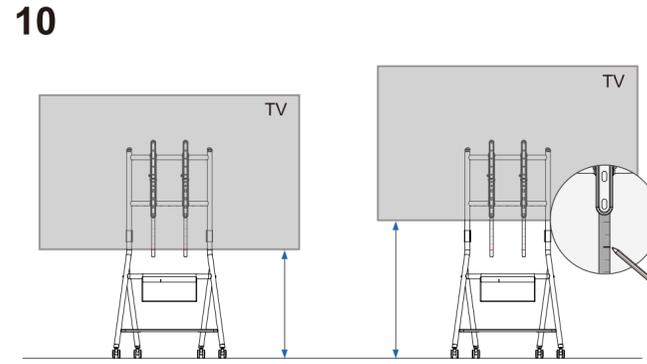
The adjustable range of the distance from the bottom of the TV to the ground is marked on the part 7, so that you can choose the appropriate height. You can choose the height, make a mark on the ruler, and then disassemble and install the part 7 to the back of the TV.
