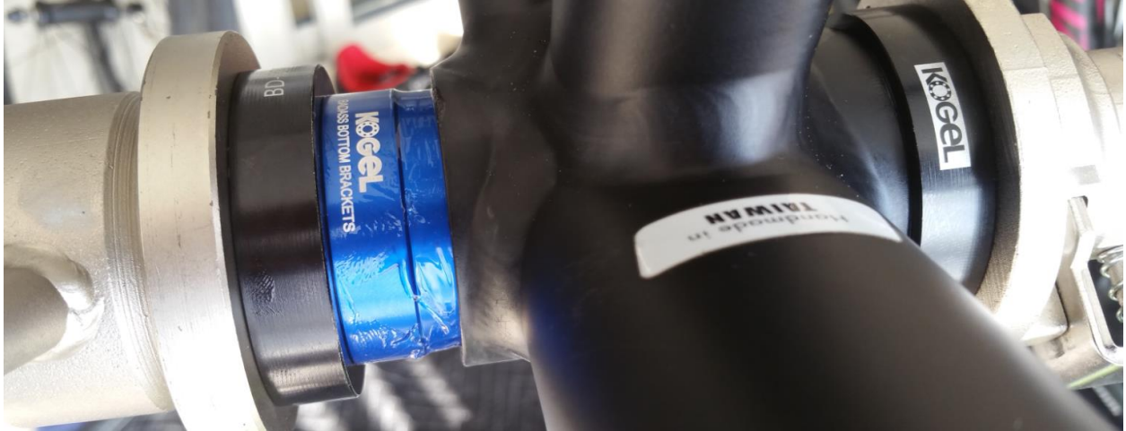
Here is a fancy new tool we developed. The Frame Guide on the right side of this photo centers the bearing press in the frame, while we press the cups one at a time.
