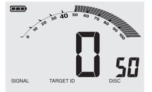
The segments along the arc will remain illuminated in this state as you are pressing  $\bigoplus$  or  $\bigoplus$ . This displays your chosen target discrimination parameter. At any time during operation, you can view the discrimination settings in one of
