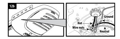
**NOTE:** After power is supplied to the powerhead: (1) Check if the red and green Safe-T-Beam<sup>®</sup> LEDs are lit. If not, return to step 9 and check wiring. (2) See if wall console red LED is lit. If not, check if a blue LED on powerhead is blinking. If yes, press the "LOCK" button on the wall console. (Wall console LED should now be lit.) Otherwise, return to step 10 and check wiring.
