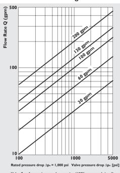
Valve flow for maximum valve opening (100% command signal) as a function of the valve pressure drop.
