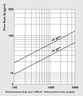
Valve flow for maximum valve opening (100% command signal) as a function of the valve pressure drop.
