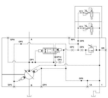
\* Be sure system and pumps are protected against over loads with a high pressure relief valve.
