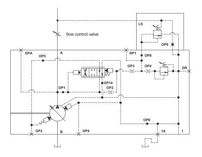
\* Be sure system and pumps are protected against over loads with a high pressure relief valve. If control shifts faster than 150 m/seconds, cavitation can occur.
