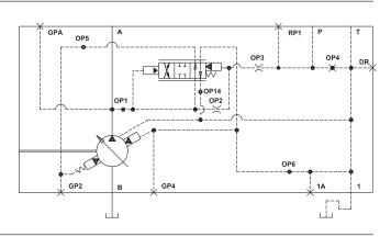
\* Be sure system and pumps are protected against over loads with a high pressure relief valve. If control shifts delivery faster than in 150 m/seconds, cavitation can occur to some degree.
