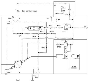
\* Be sure system and pumps are protected against over loads with a high pressure relief valve. If control shifts faster than 150 m/seconds, cavitation can occur.
