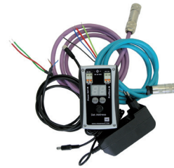
Figure 3. R-Series Profibus-DP Handheld Address Programmer, part no.: 280640
