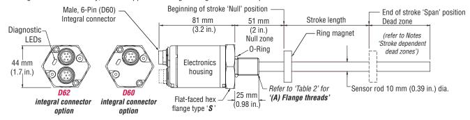
Figure 7. Model RH Rod-style sensor dimension reference (shown with D60 / D62 integral connector options)
