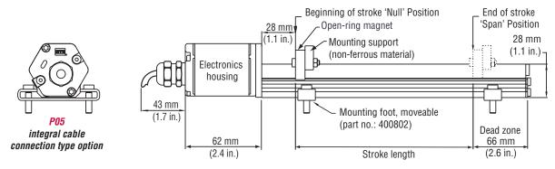
Figure 5. R-Series Model RP Profile-style sensor dimension reference (Shown with the **P05** integral cable option)
