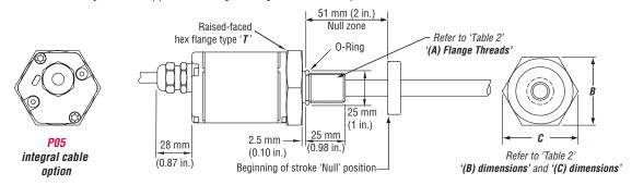
Figure 8. Model RH Rod-style sensor dimension reference (shown with *P05* integral cable option)
