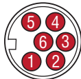
Male, 6-pin (D60) integral connector pin-out as viewed from the end of the sensor
