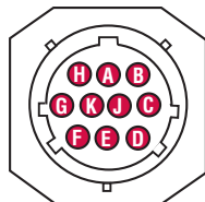
Male, 10-pin in-line or integral MS connector (Option FM_ or MS0)
