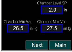
Set-point screens allow the viewing and modification of temperature, level, vacuum, timer, and alarm set-points.
