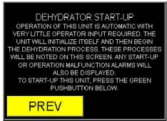
Start-up screens guide first-time users through a five step checklist to verify that proper utility connections have been made.
