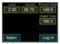
A three-step automated startup begins when the "START" push button is pressed. The main screen appears automatically when dehydration begins.
