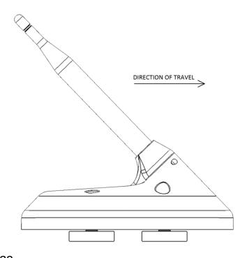
The power cable from unit will protrude from the bottom of the unit and the magnetic mounts provide sufficient clearance for the cable. The area where the cable makes entry into the unit has been weatherproofed to ensure compliance with IP67 moisture and dust penetration standards.
