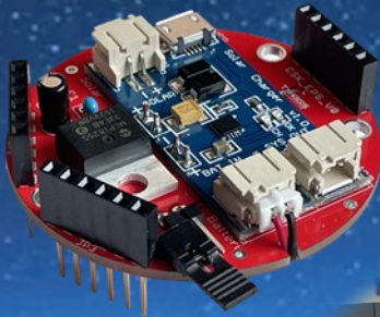
Electrical Power Subsystem (EPS)
