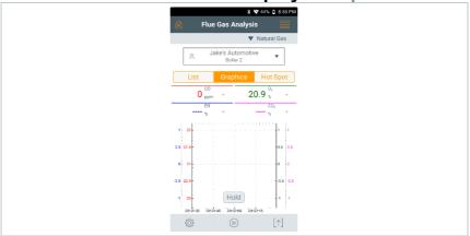
In the Main measurement display - **Graphics**, the reading progression can be displayed as a line diagram.
