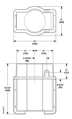
Figure 23. Dimensions of 599-10065 SKB\C Weather Shield in Inches (Millimeters).
