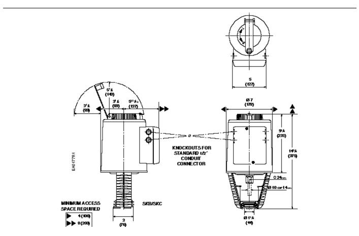
Figure 25. SKB/C Weather Shield, 599-10071 in Inches (Millimeters).
