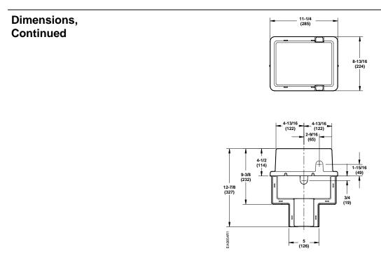
Figure 24. Dimensions of 599-10071 SKD Weather Shield in Inches (Millimeters).
