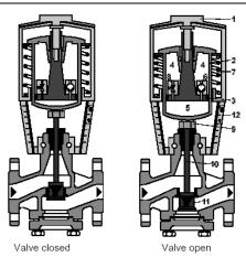
Figure 6. SKB/C Valve Parts.
