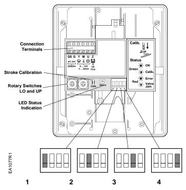
Figure 13. DIP Switches.
