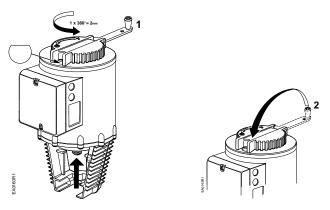
Figure 17. SKB/C Automatic Operation.
