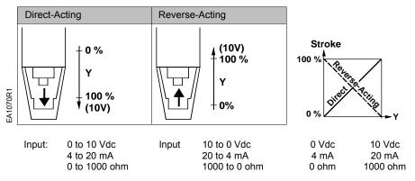
Figure 14. Direction of Operation.
