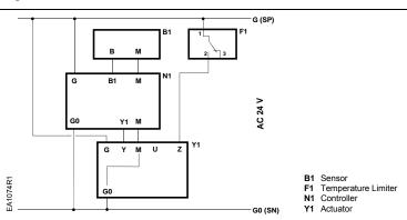
Figure 19. Terminal Connections.
