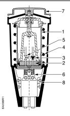
Figure 7. SKD Valve Parts.
