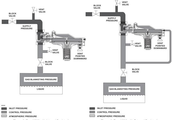
Figure 2. Type Y692 with Internal Registration Operational Schematic
