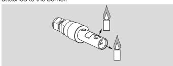
The UV tube can be directed towards the flame from the side or front with the help of the viewing openings in the sensor head.
