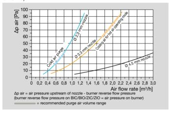
A purge air nozzle is not required for Kromschröder burners (BIO, BIC, ZIO, ZIC) if they are used with cold combustion air.
