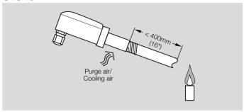
The sensor is mounted to a 1/2" viewing tube using the adapter (supplied) with integrated quartz glass heat guard. The viewing tube should be directed at the first flame third, as this is where the highest UV radiation is generally found. The inside of the steel tube should not be coated.
