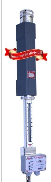
**FLO-TRONIC Plus™** is based on a standard *FLO-METER™* with or without a manual flow control valve. The *FLO-TRONIC Plus™* provides visual flow rate indication as required by NFPA as well as an analog output in direct relation to the flow rate.
