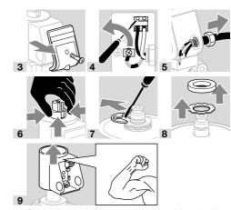
→ Depending on the construction stage of the unit, there are two different methods for replacing the actuator: If the unit concerned has no O-ring in this place (arrow), replace the actuator as described here. Otherwise, go to the next note.
