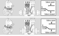
→ When installing two plugs on a VAN with closed position indicator: label the sockets and plugs to avoid confusion.
