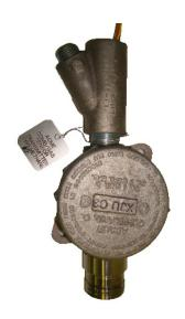
he Acme Combustible gas sensor-transmitter measures the concentration of the target gas in an enclosed area and produces a proportional analog output signal.
