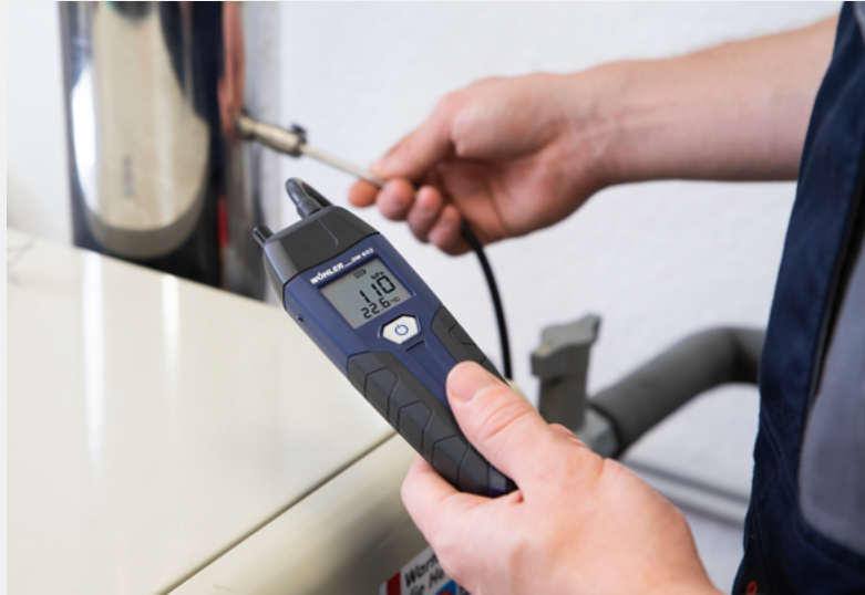
The Wohler DM 602 is a fast and precise tool to adjust burners and measure chimney drafts.
