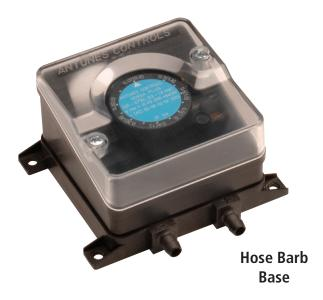
The Versa Plus Air is a highly accurate air pressure switch that monitors positive, vacuum, or differential air pressure. The integrated contacts make or break circuits to a desired setpoint. The omega spring design provides repeatability and accuracy. It is compact, easy to install, and available in various mounting configurations.
