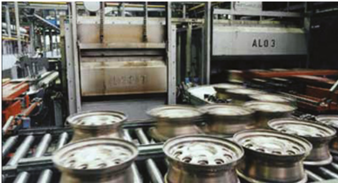
Aluminium industry: curing oven for wheel rims
