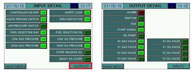
When the LMV controller is in alarm, the ALARM output will flash bright red. When the controller is not in alarm, the alarm output will be a dull red background. All other outputs that are currently active will display as ON with a bright green background. All other outputs that are currently inactive will display as OFF with a dull green background.
