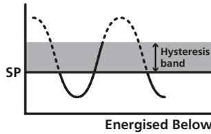
**CNTRL - SETPOINT VALUE** controls setpoint deactivation point. **HYSTERESIS VALUE** controls setpoint reactivation point.
