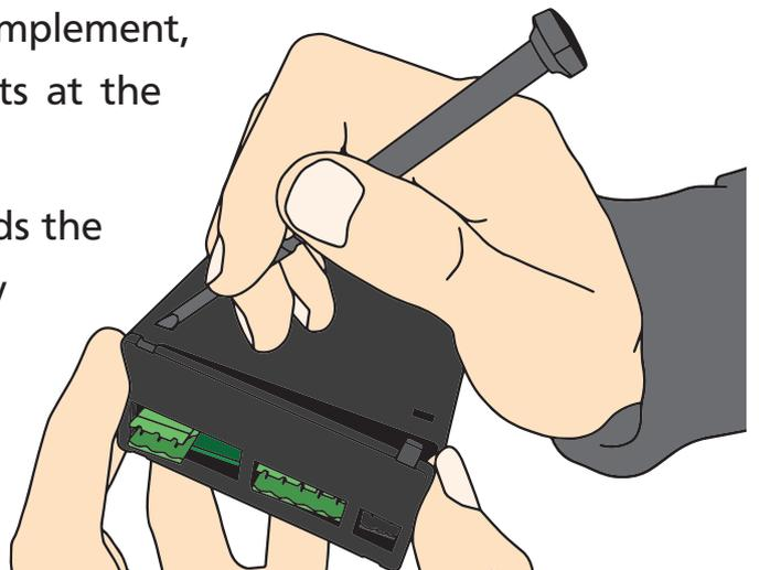
**D** You should now be able to remove the back plate. If it does not unclip easily, you may need to disengage the two remaining tabs by repeating steps 5.2B–C on the other side of the meter.
