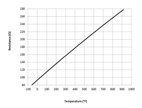
Pt1000, 385 characteristic (QAE2012.001, 544-577-25, 544-577-40, 544-577-60, QAE2012.9002, QAM-P206, QAM-P210, QAM-P224)
