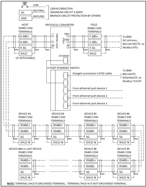
ProtoNode TS-PX4-6-8 Port Ethernet Switch (BACnet/IP, BACnet MS/TP, Ethernet/IP, N2 Johnson, or Modbus RTU)
