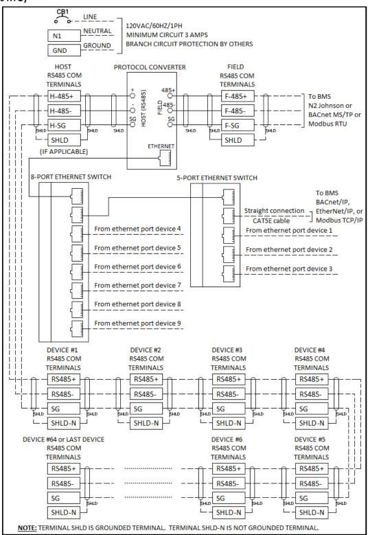
ProtoNode TS-PX4-12-16 Port Ethernet Switch (BACnet/IP, BACnet MS/TP, Ethernet/IP, N2 Johnson, or Modbus RTU)
