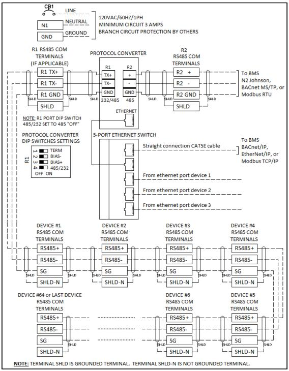
ProtoAir TS-PX4-6-8 Port Ethernet Switch (BACnet/IP, BACnet MS/TP, Ethernet/IP, N2 Johnson, or Modbus RTU)
