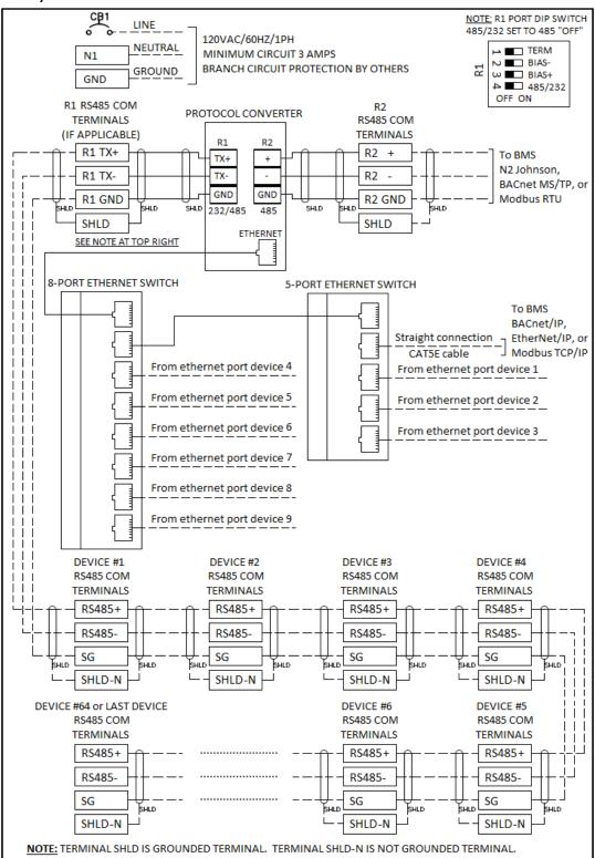
ProtoAir TS-PX4-12-16 Port Ethernet Switch (BACnet/IP, BACnet MS/TP, Ethernet/IP, N2 Johnson, or Modbus RTU)
