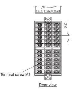
Terminal block is not attached to unused terminals (terminal 13 to 24) according to the model.
