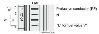
Figure 27: Fuel valve V1 terminal X7-04
