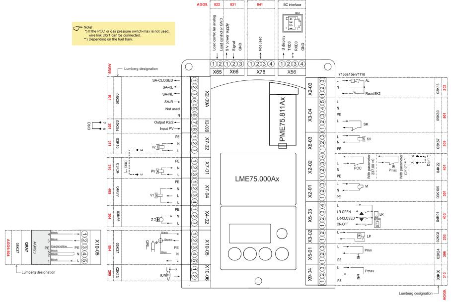
Figure 29: LME75.000Ax: Inputs and outputs / internal connection diagram
