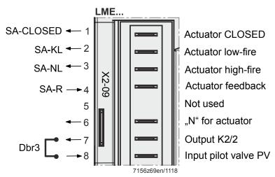
Figure 18: Output for actuator terminal X2-09
