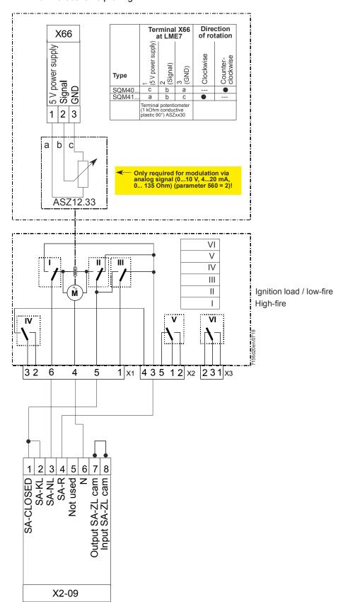
Figure 22: Connection diagram example 1: LME75.000Ax with SQM40/SQM41 (diagram 8) and ASZ
