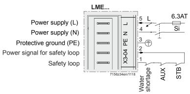
Figure 15: Safety loop terminal X3-04
