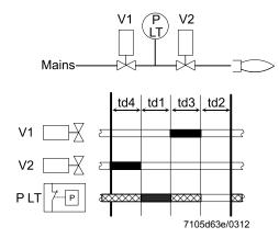
Figure 10: Valve proving with separate pressure switch
