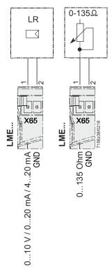
Figure 13: Analog input for load controller terminal X65
