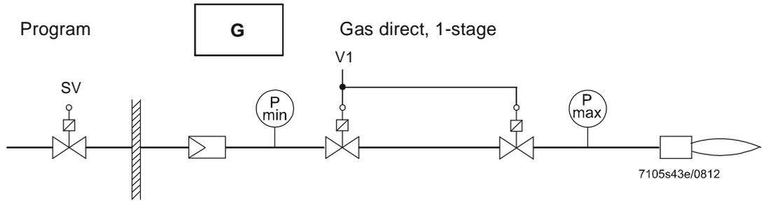
Figure 2: Fuel train gas direct ignition (G), 1-stage
