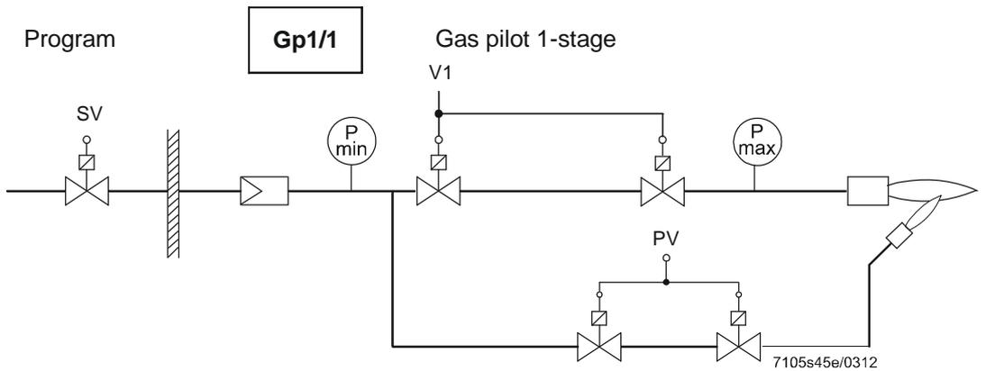
Figure 3: Fuel train gas pilot ignition 1 (Gp1/1), 1-stage
